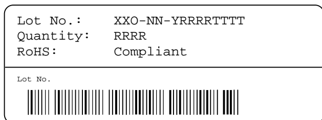
Figure 12: First label on reel: XX = Sensor Type (21 for SHT21), O = Output mode (D = Digital, P = PWM, S = SDM), NN = Chip Version, Y = last digit of year, RRRR = number of sensors on reel, TTTT = Traceability Code.
